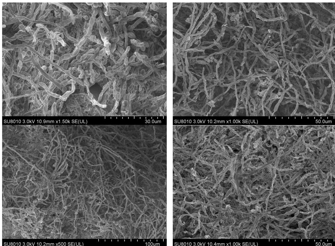
Figure 4: SEM of biofilm during stable operation.
