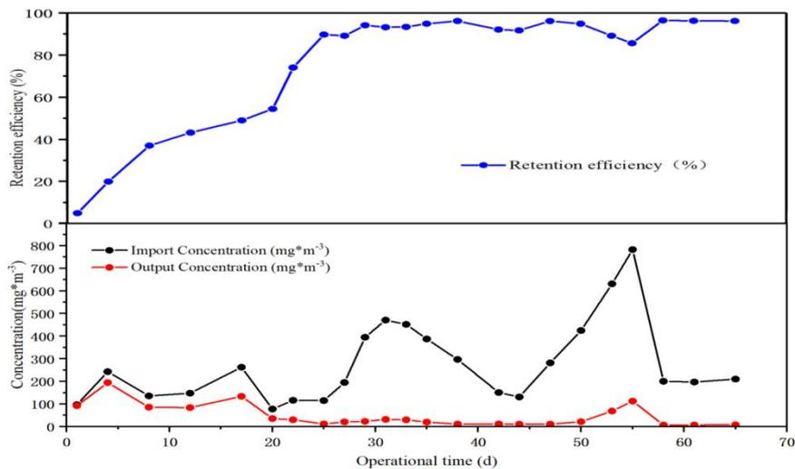
Figure 3: Performance of toluene removal efficiency during stable operation.
