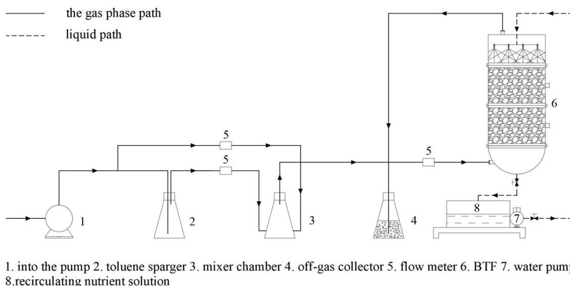
Figure 1: Process flow chart of biological filtration system.
