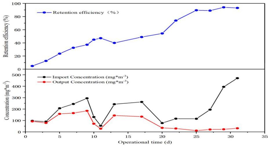
Figure 2: Change of degradation rate of toluene during biofilm culturing.
